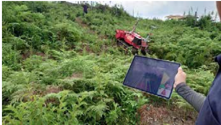
Verification test (automated weeding machine climbing up a field with an angle of about 25 degrees)
